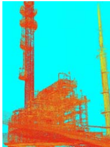
3D PlantLINx Software Converting Laser scans into 3D models
